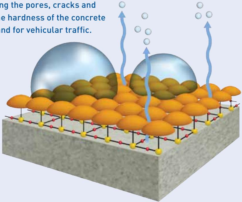
The resulting denser mass is solid, colorless, odorless, non-toxic (no VOCs) and non-flammable. Water, chemicals and other contaminants can no longer penetrate into the concrete.
